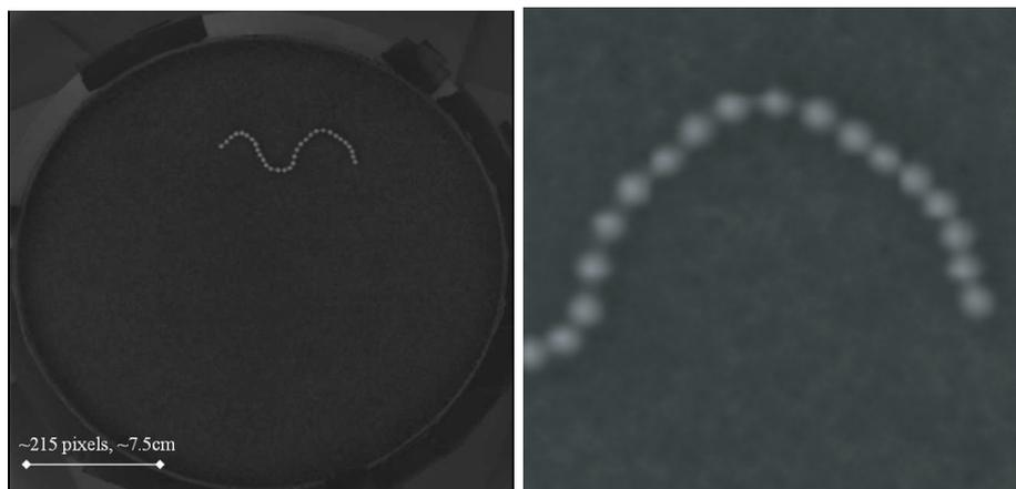
Figure 3: Image and blowup of 32 bead long chain. One bead diameter is approximately 6-8 pixels.
