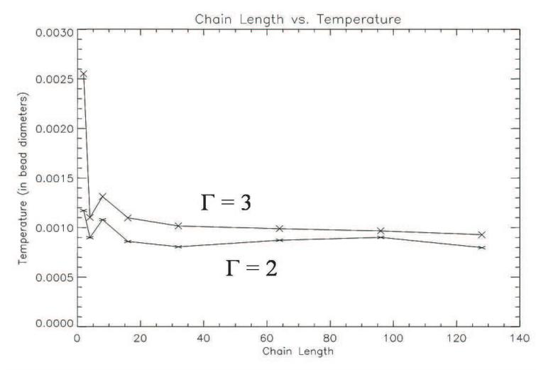
Figure 11: Temperature is independent of chain length and dependent on acceleration in the limit of  $N \gg 1$ .
