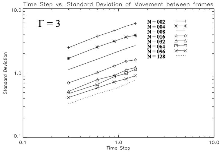
Figure 9: A diffusion constant can be determined from the slopes of each of these lines.
